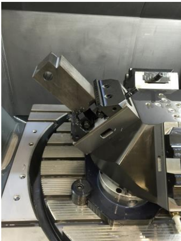
6-jaw in use for high-strength materials
